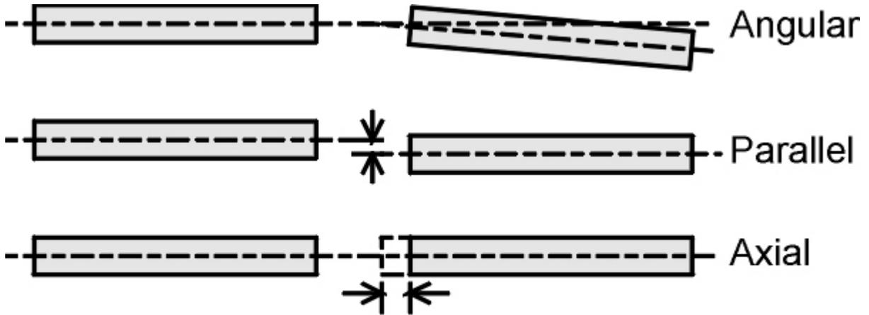
**Fig 4.2 Alignment Errors**
