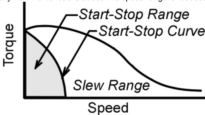
**Fig 2.7 Slew Curve**
