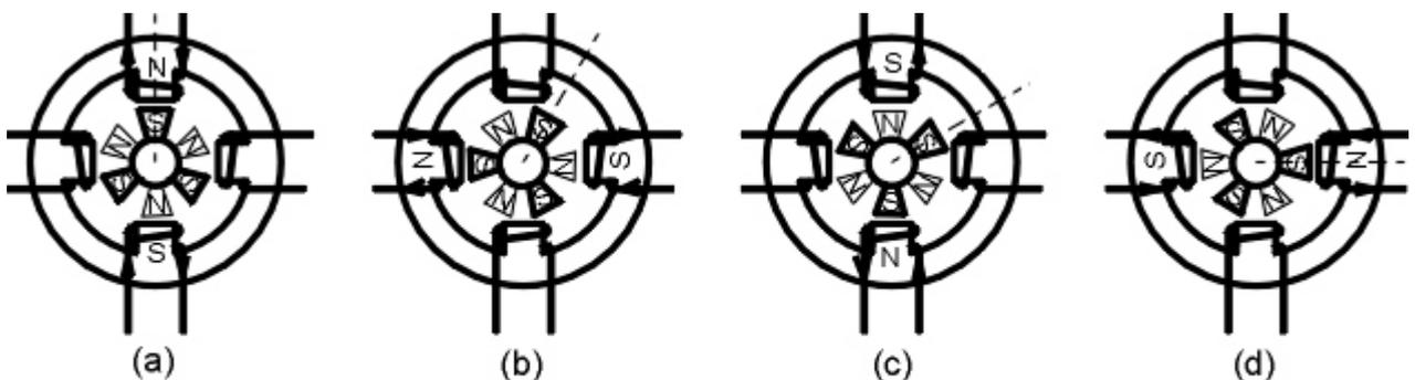
**Fig. 2.2 Full Stepping, one phase on**
