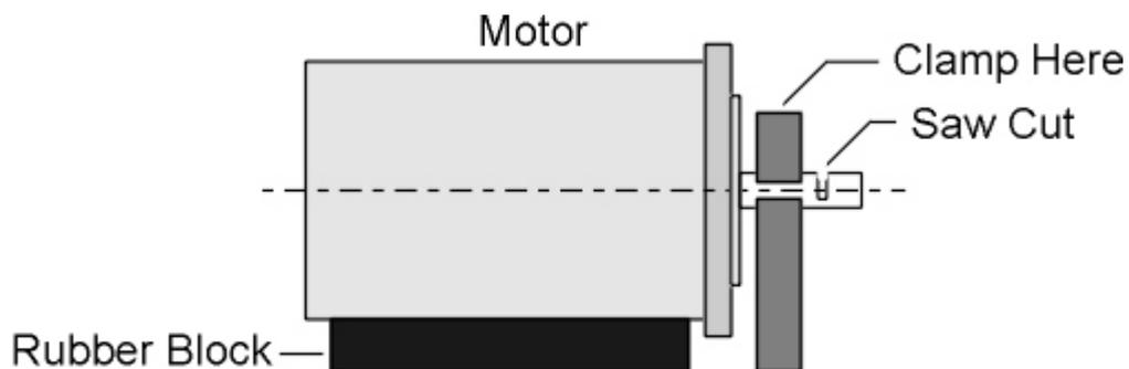
**Fig 4.6 Shortening Motor Shaft**
