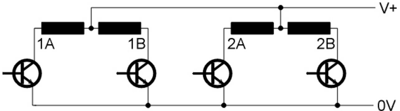
**Fig. 3.2 Basic Unipolar Drive**
