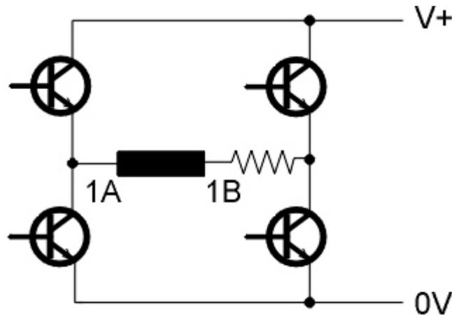
**Fig. 3.4 Bipolar Drive (one winding shown only)**
