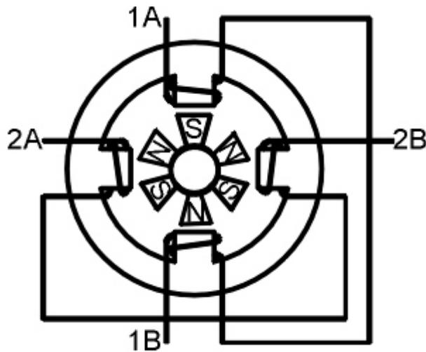
**Fig. 2.1 Simple Hybrid Stepper Motor**
