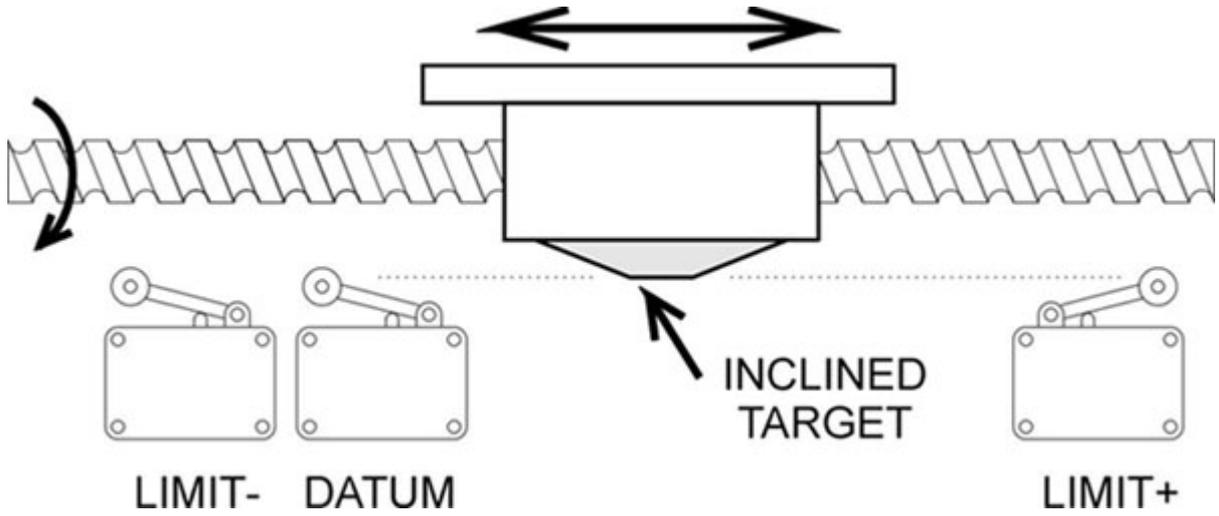
Fig. 5.11 Limit Switch Ramps
