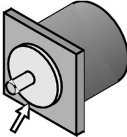
**Fig 4.1 Motor Pilot Register**
