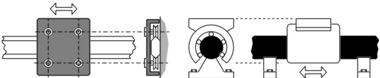
Fig. 5.8 Linear Bearings
