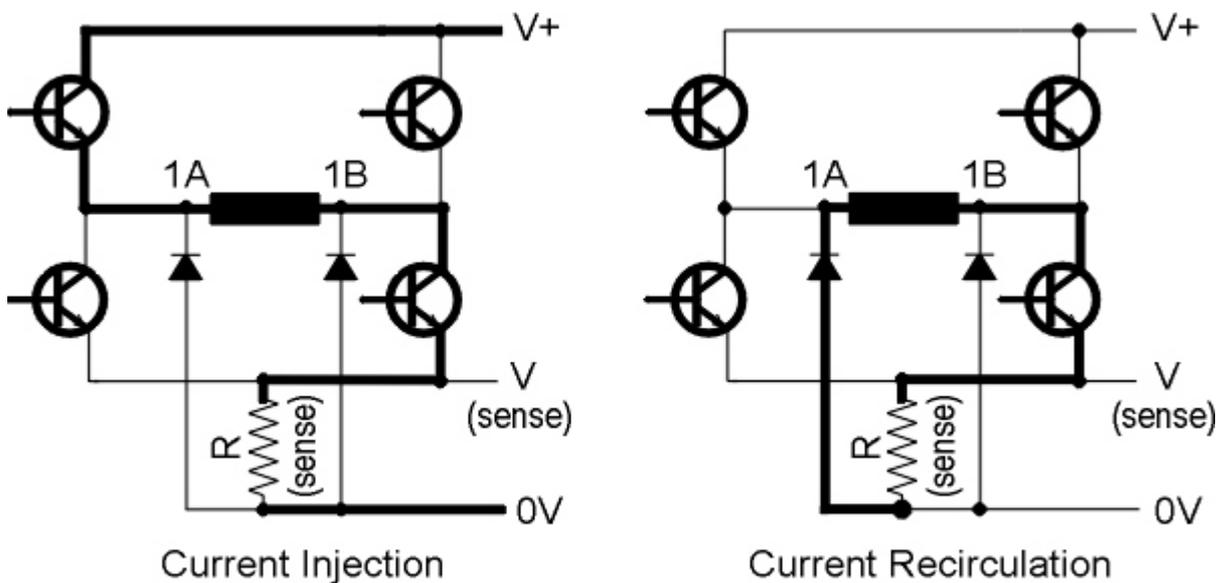
**Fig. 3.5 Recirculating Chopper Drive (one winding shown only)**
