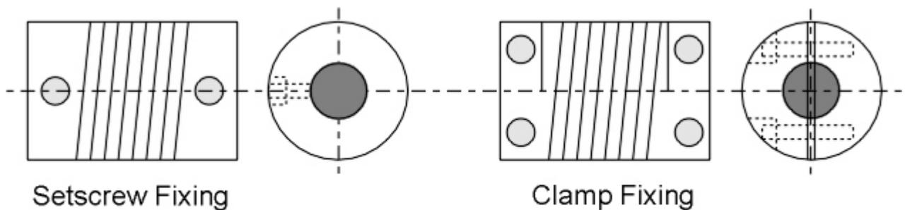
**Fig 4.3 Coupling Fixing**
