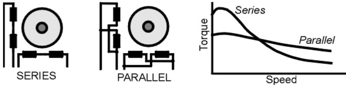
**Fig. 2.6 Series and Parallel Connections**
