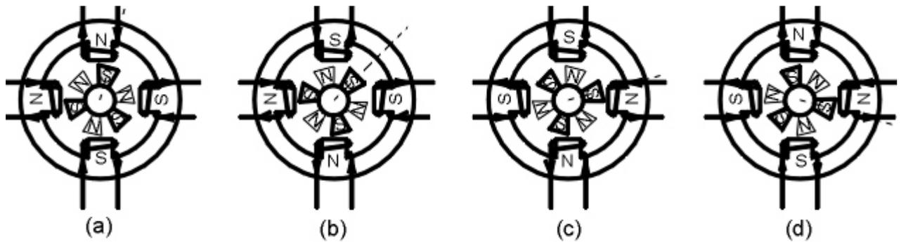
**Fig. 2.3 Full Stepping, two phases on**
