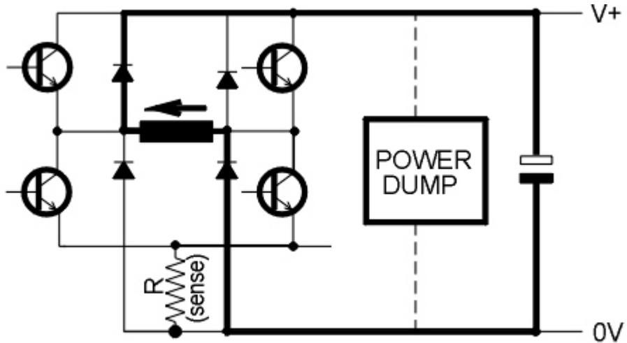
**Fig. 3.6 Current Flow During Regeneration (one winding shown only)**
