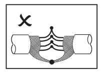
There should be no break in the  $360^{\circ}$  coverage that the screen provides, except at ends. If a connector must be used, it should be metallic and maintain  $360^{\circ}$  coverage of the screen. If cables must be joined, a metallic junction must be used and earthed.
