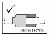
Lock the ferrite onto the cable by fitting some 19mm diameter heatshrink over it and shrinking it onto the cable. If heat shrink is not available, use cable ties but these will give no protection to the ferrite..
