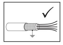
Use metal braided screened cables. Connect the screen to ground (0V common).
