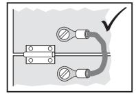
Hinged doors must also be earthed as there may not be low resistance path through the hinge. Most enclosures are supplied with threaded copper earthing studs for this purpose.
