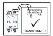
Mount the filter as close as possible to the transformer.
