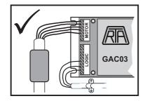
Locate the ferrite core next to the drive but inside the enclosure.
