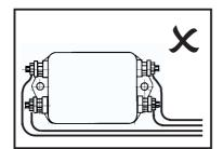
When connecting, keep the input cables away from the output cables.
