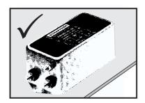
Filters must be mounted on a conductive base plate. Leakage currents can be very high so earthing is important. If the base plate is painted or powder coated, remove the coating from where the mains filter is going to be located.
