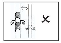
Route control cables away from motor and power cables.
