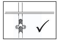
Avoid crossing power or motor cables with control cables, but if you must do this, do so at  $90^{\circ}$  to avoid EMI pickup.
