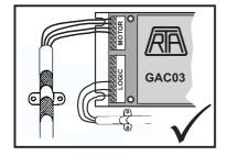
Within the cabinet, all motor cables should lie in the same trunking. They should be separated from low level control signals. Control signals should also be separated from power cables.
