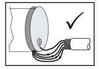
Stepper motors with terminal boxes are better for EMC compliance, but are much more expensive. If motors with unscreened flying leads are used, join these leads to the braided screened cable within 100mm of the motor. Most stepper motors have an earth screw for the earth connection. Connect the earth conductor in the cable to this screw.
