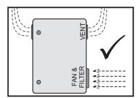
It is still necessary to ensure the drives and transformer all have adequate cooling. Filters may be needed on fans to ensure dust and metal particles do not enter the enclosure.
