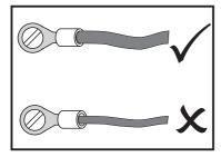
Use low impedance conductors for earth lines. Thin cables have higher resistance than thick cables.
